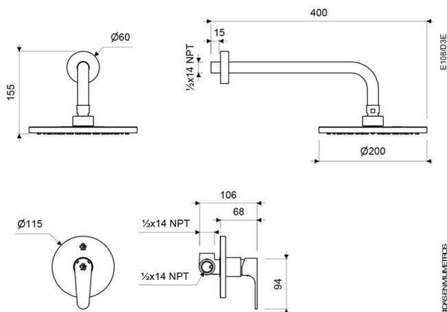
MEASUREMENTS IN MILLIMETERS
